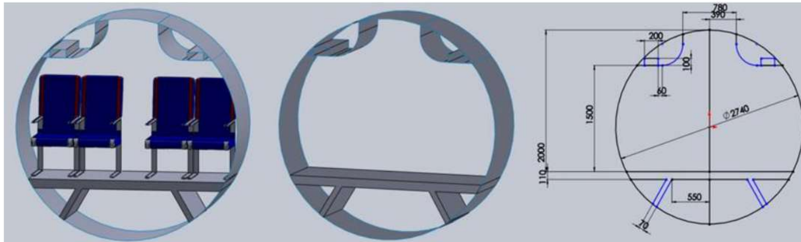
Fig. 2 CAD model of the fuselage trunk (dimensions are given in [mm])
